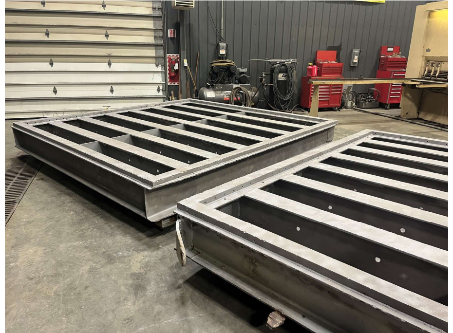
Valve Bulkheads Being Repaired
